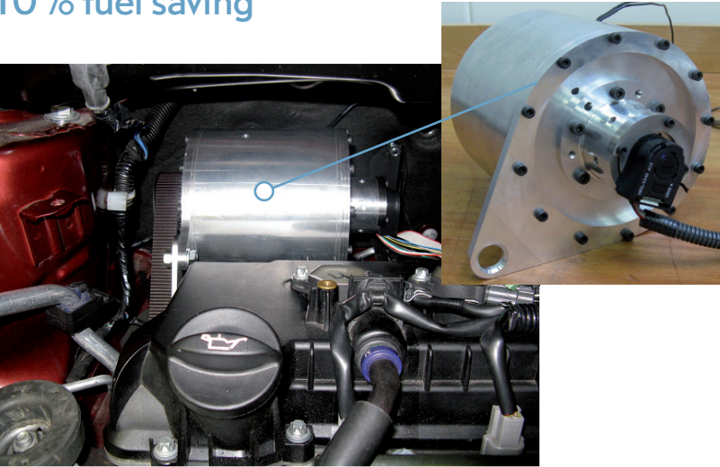
Electrically charged flywheel module
